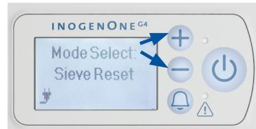
12. Press and hold the plus (+) and (-) minus button for 5 seconds. The screen will display “sieve reset” message. Release button once message is displayed on screen.
