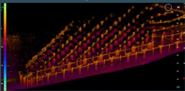
This data set illustrates the ability of the Echoscope to penetrate and image complex structures with high point density and multiple angles of incidence reducing acoustic shadowing and providing comprehensive coverage.
