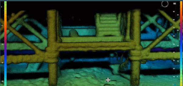
This data set was collected as a real-time, fully geo-referenced mosaic with RTK positioning in <u>less than</u> <u>1 minute of survey time</u>. The 3D point cloud density and the volumetric aperture provide comprehensive coverage of the pier and surrounding environment allowing the user to easily identify the state of the structure and any localised debris
