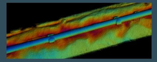
This data set illustrates the ability of the Echoscope to provide coverage of the pipeline with high point density enabling the user to monitor general status and highlight areas of interest such as scour zones causing freespan.
