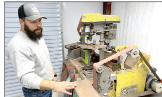
Adam Thomas of Goose Creek Knives inspects his 2-inch-by-72-inch belt grinder, used for shaping and sharpening knife steel.
