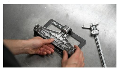
With Stratasys and trinckle's software technology, a precision metrology inspection fixture that securely positions parts for accurate measurement. The 3D-printed design eliminates costly machining while maintaining tight tolerances.
