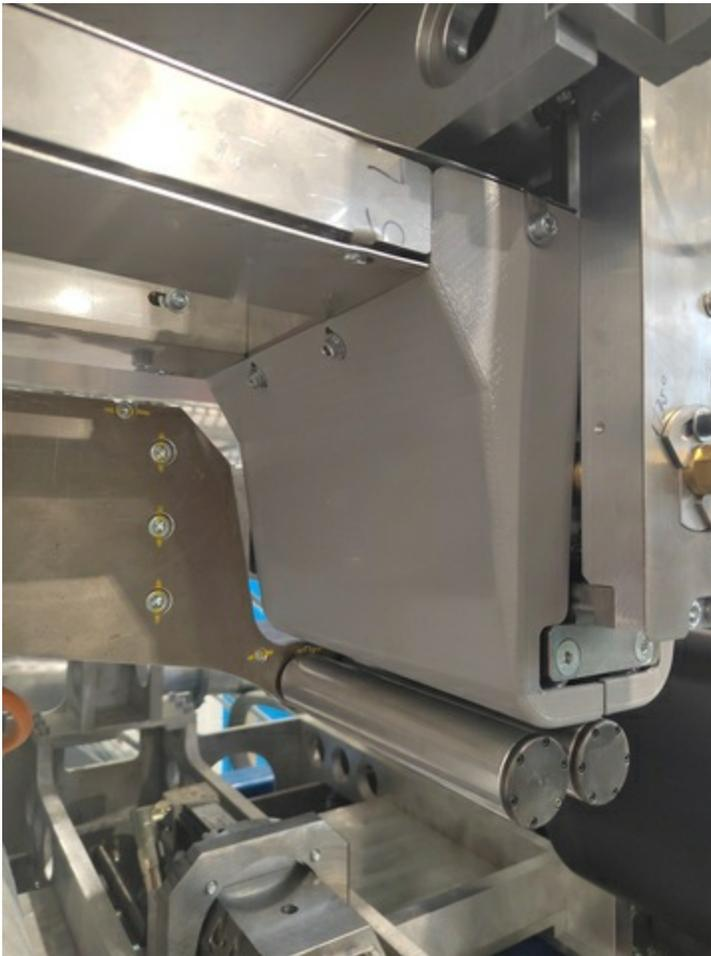
A 3D-printed protection cap, taking the place of an original aluminum part that wasn't fitting properly. With 3D printing the company was able to do several iterations and find the best fit possible. (Photo: Business Wire)
