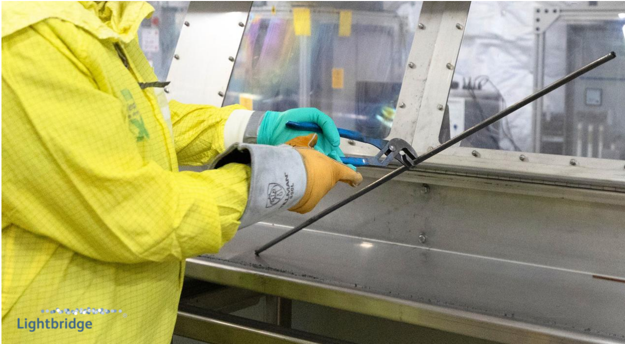
URANIUM-ZIRCONIUM ROD POST-EXTRUSION:
