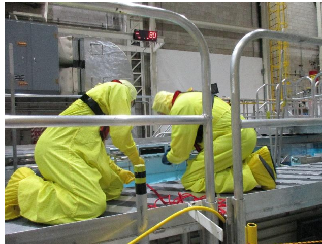
Loading of one of the capsules into an experimental assembly in the ATR canal.
