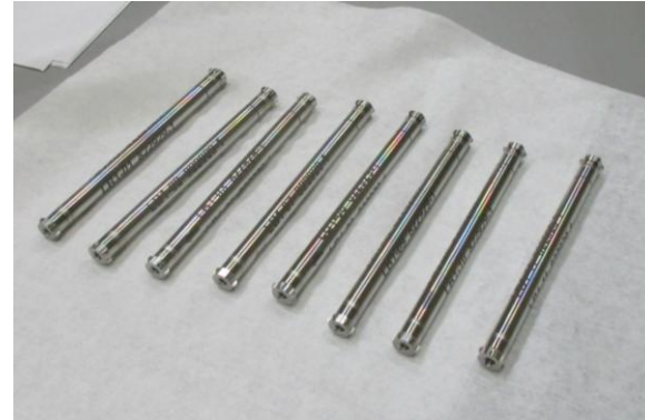
Capsules containing Lightbridge Fuel material samples before loading into an experimental assembly.
