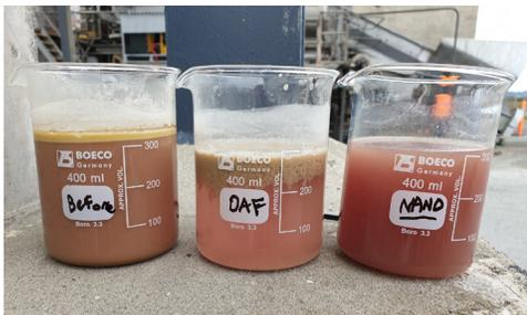
*The impact of the nanobubble treatment is clearly visible in the samples.*
