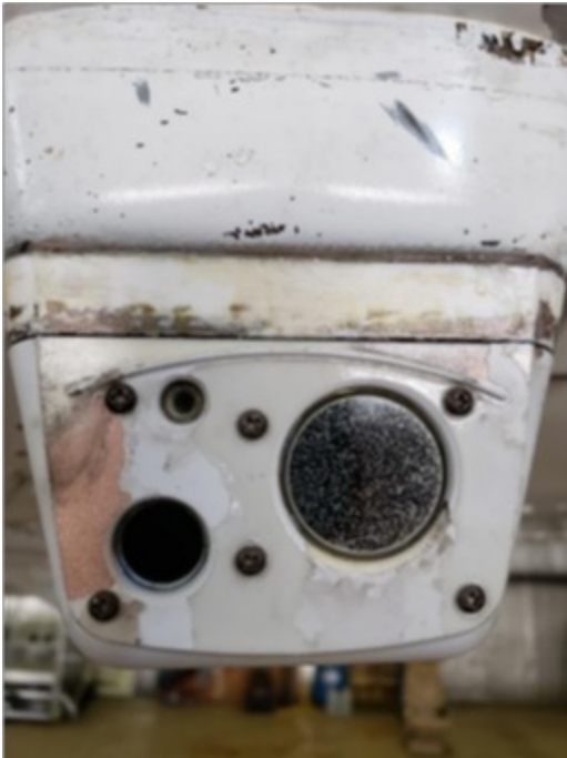
Astronics' Max-Viz sensor installation still operated perfectly under the Caravan wing after 6,000 hours and 1.1. million miles, but shows some cosmetic wear and tear.
