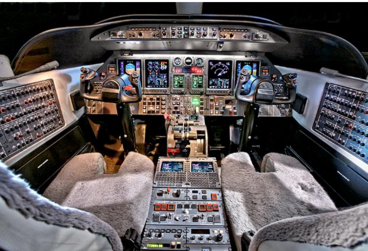
Traditional Cockpit with Mechanical Circuit Breakers Learjet 45
