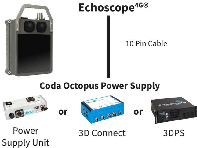
These Data Integration Units support Time Sync feature specifically for standard Echoscope sonar
