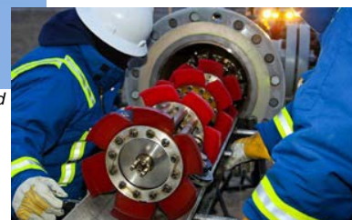
Pipelines deliver massive amounts of crude daily and ensuring safe operation is key. The EMCORE TAC-450-DSP1750, coupled to additional sensors, provides these inspection robots with extremely accurate angular data.
