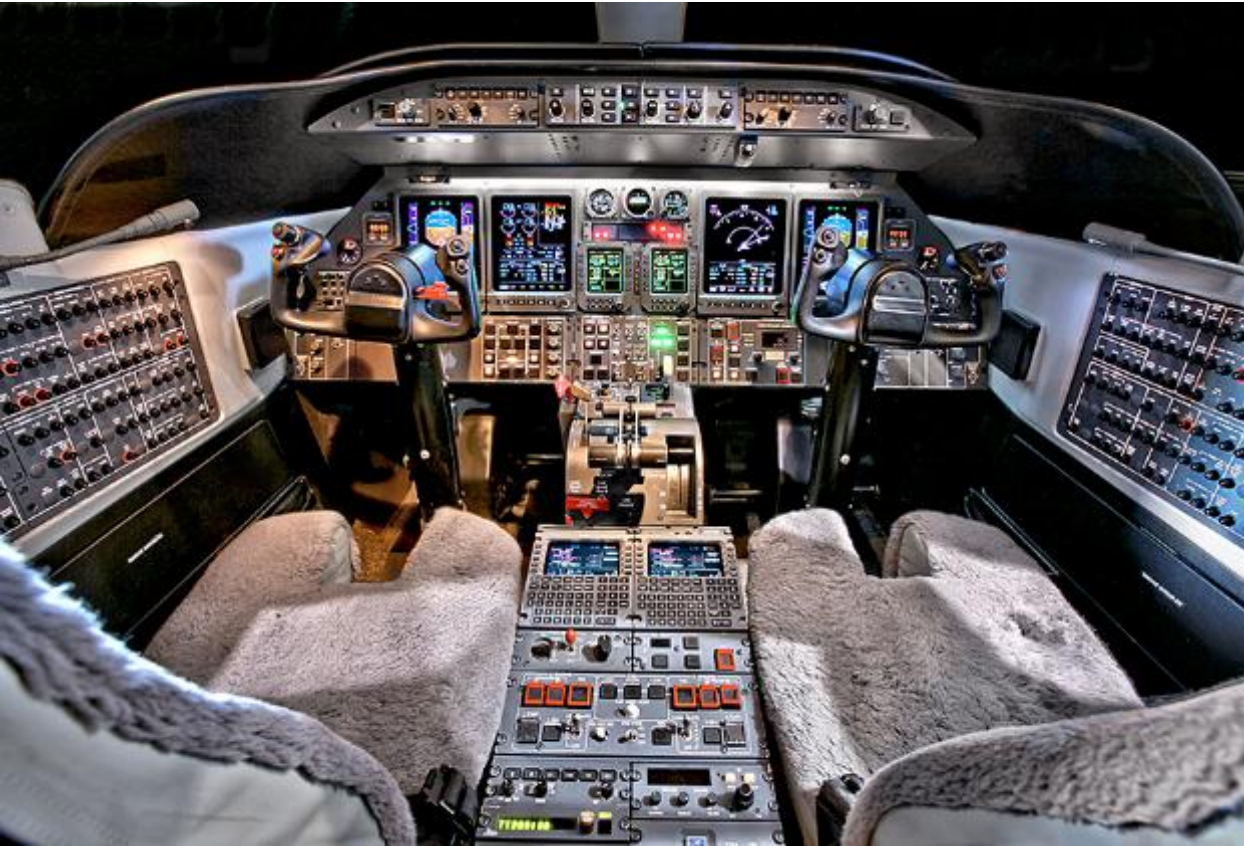
Traditional Cockpit with Mechanical Circuit Breakers Learjet 45
