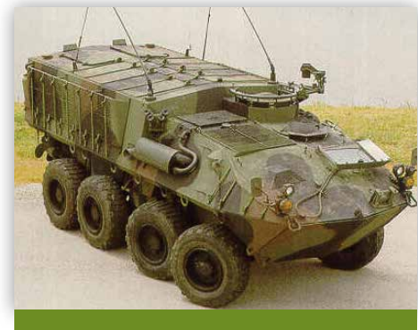
The U.S. Army “Stryker” armed personnel carrier uses armor plate produced with FINELINE® processing for improved toughness and spalling resistance.
