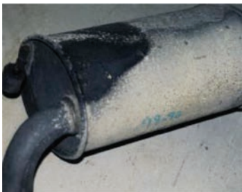
Aluminized 409 after 10 years in Windsor, Ontario, Canada. Black on the muffler top and tailpipe is paint.
