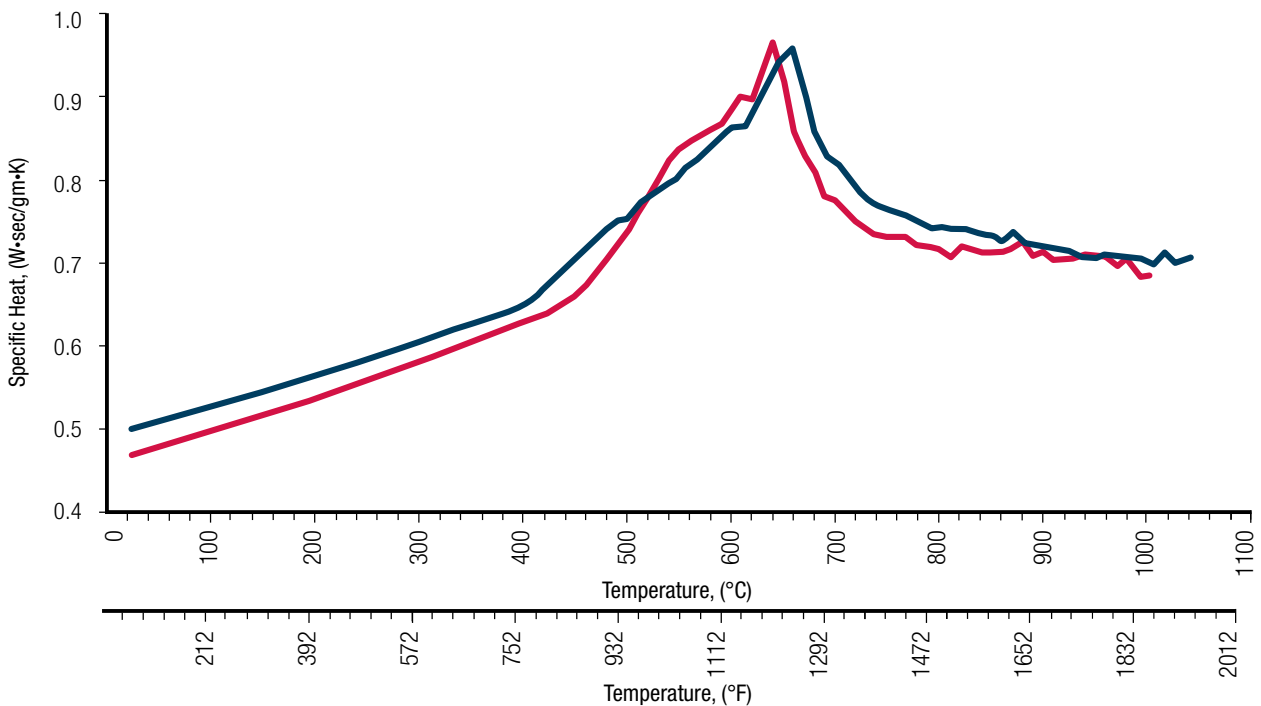
FIGURE 2 – SPECIFIC HEAT VS. TEMPERATURE
