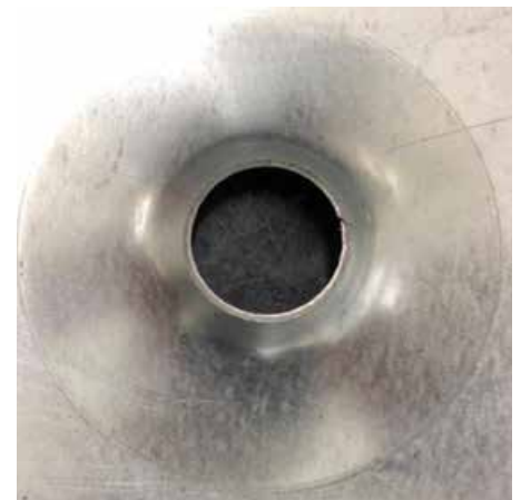
780CP Hole expansion test
