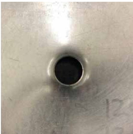
780DP Hole expansion test
