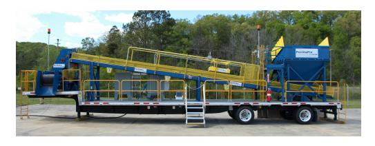
The Perma-Sort<sup>SM</sup> conveyor-based radiological assay system
