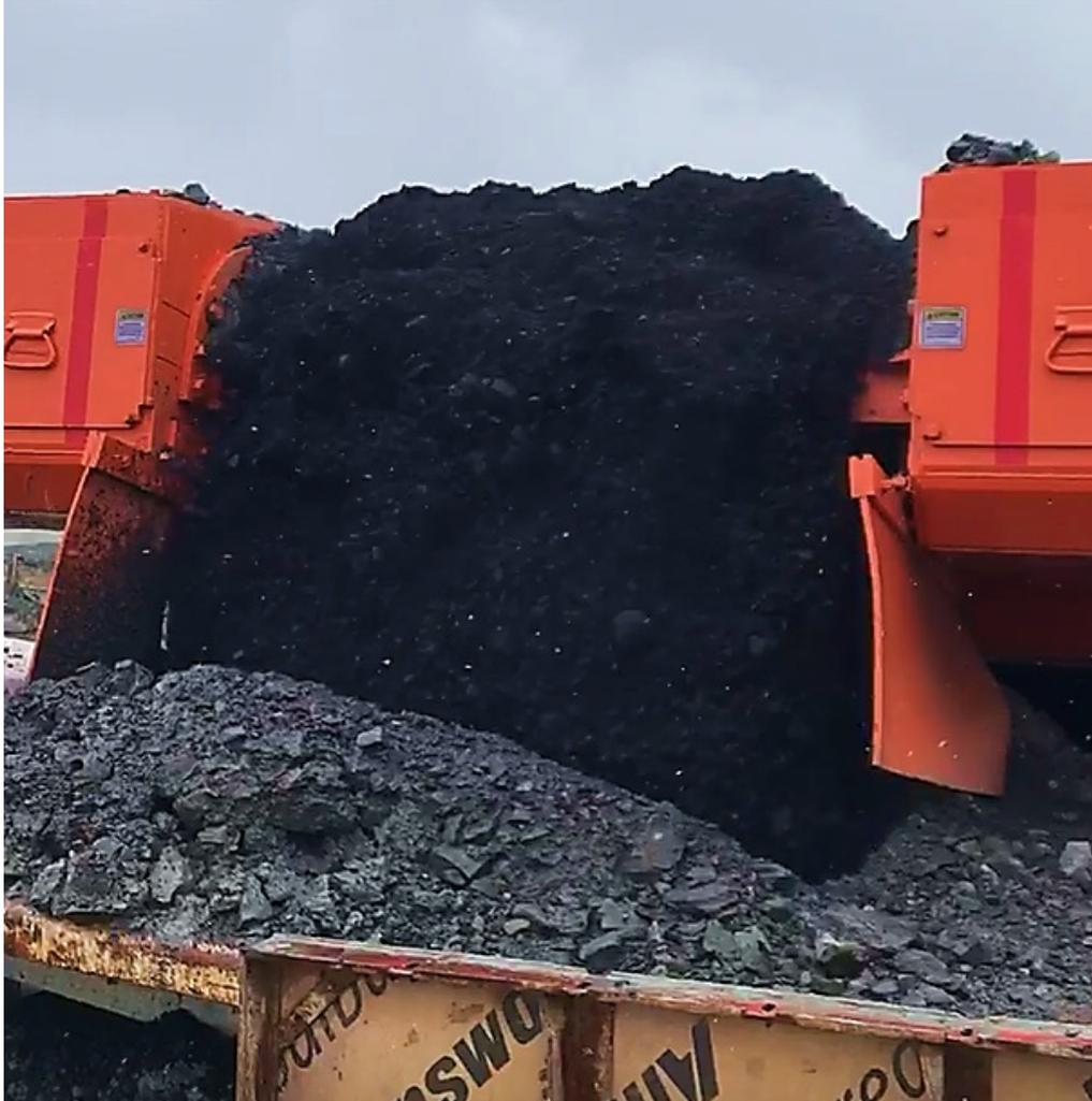
***Figure 1: Surface feeder transferring coal from the Poplar Grove mine to the CHPP
