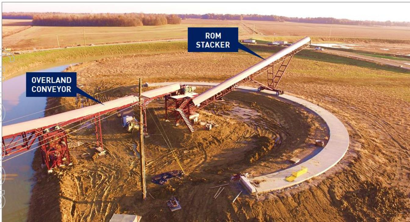
**Figure 2: ROM stacker complete and ready to stack raw coal for processing at the CHPP**
