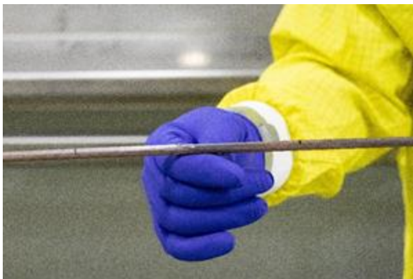
Close-up View of the Enriched Uranium-Zirconium Rod Post-Extrusion, still covered in the extrusion lubricant
