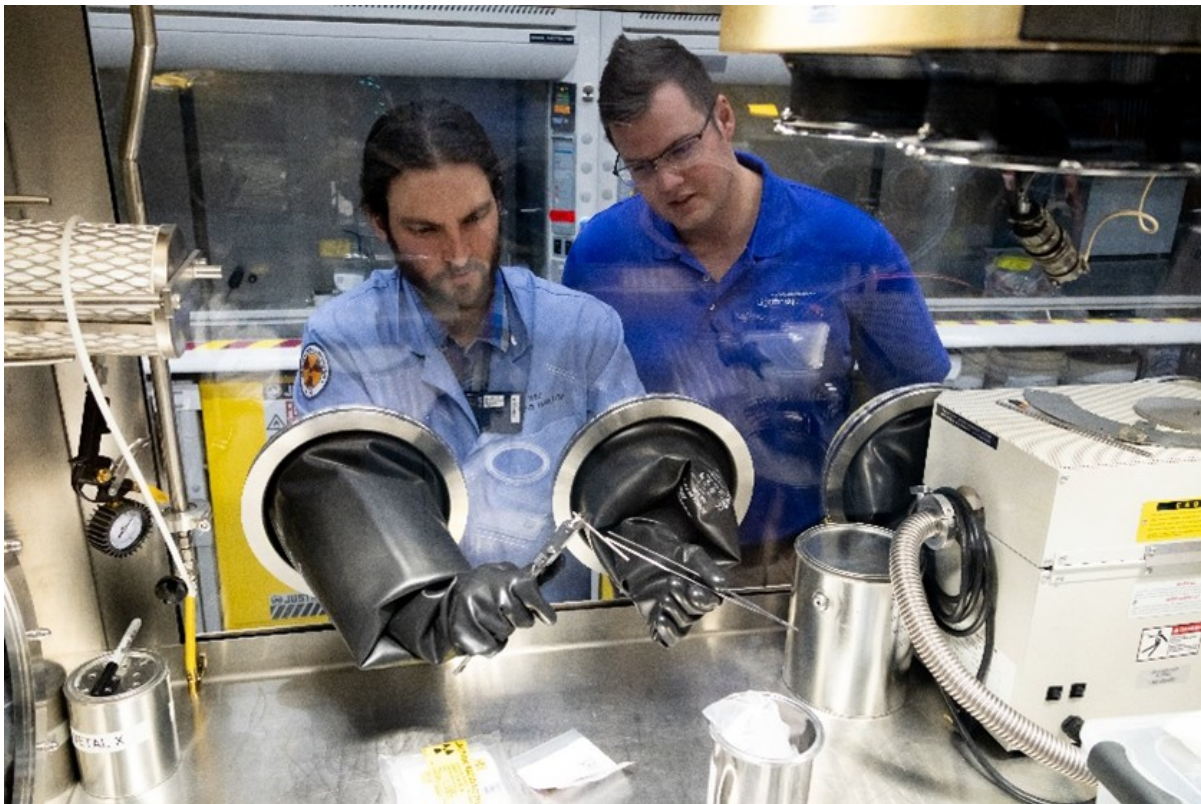
Image 5: Lightbridge and INL team performing a visual inspection of a finished enriched uranium-zirconium coupon sample inside a glovebox
