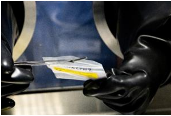
A close-up view of a finished enriched uranium-zirconium coupon sample
