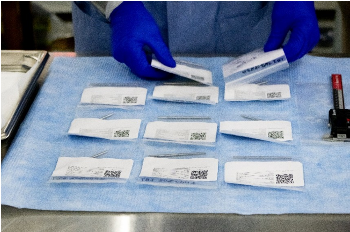
Image 8: Finished enriched uranium-zirconium coupon samples after characterization and visual inspection results confirmed their suitability for irradiation testing in the Advanced Test Reactor
