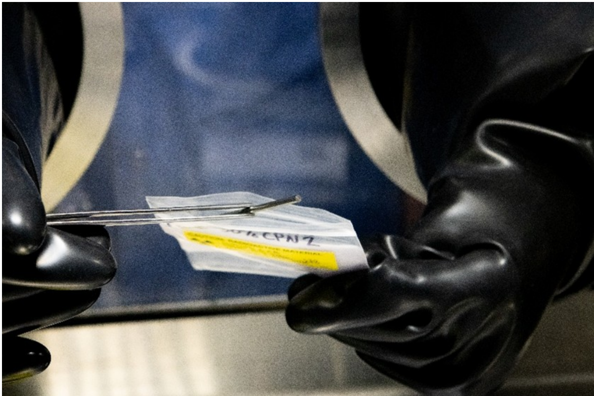
Image 6: A close-up view of a finished enriched uranium-zirconium coupon sample
