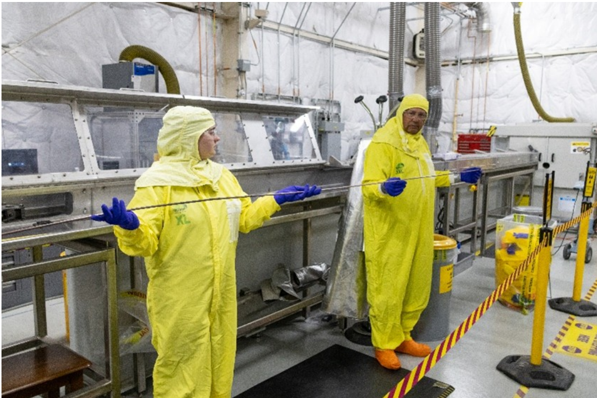
Image 1: Enriched Uranium-Zirconium Rod Post-Extrusion
