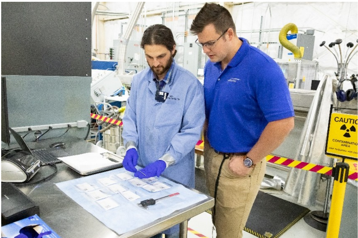
Image 9: INL and Lightbridge team inspecting the finished enriched uranium-zirconium coupon samples
