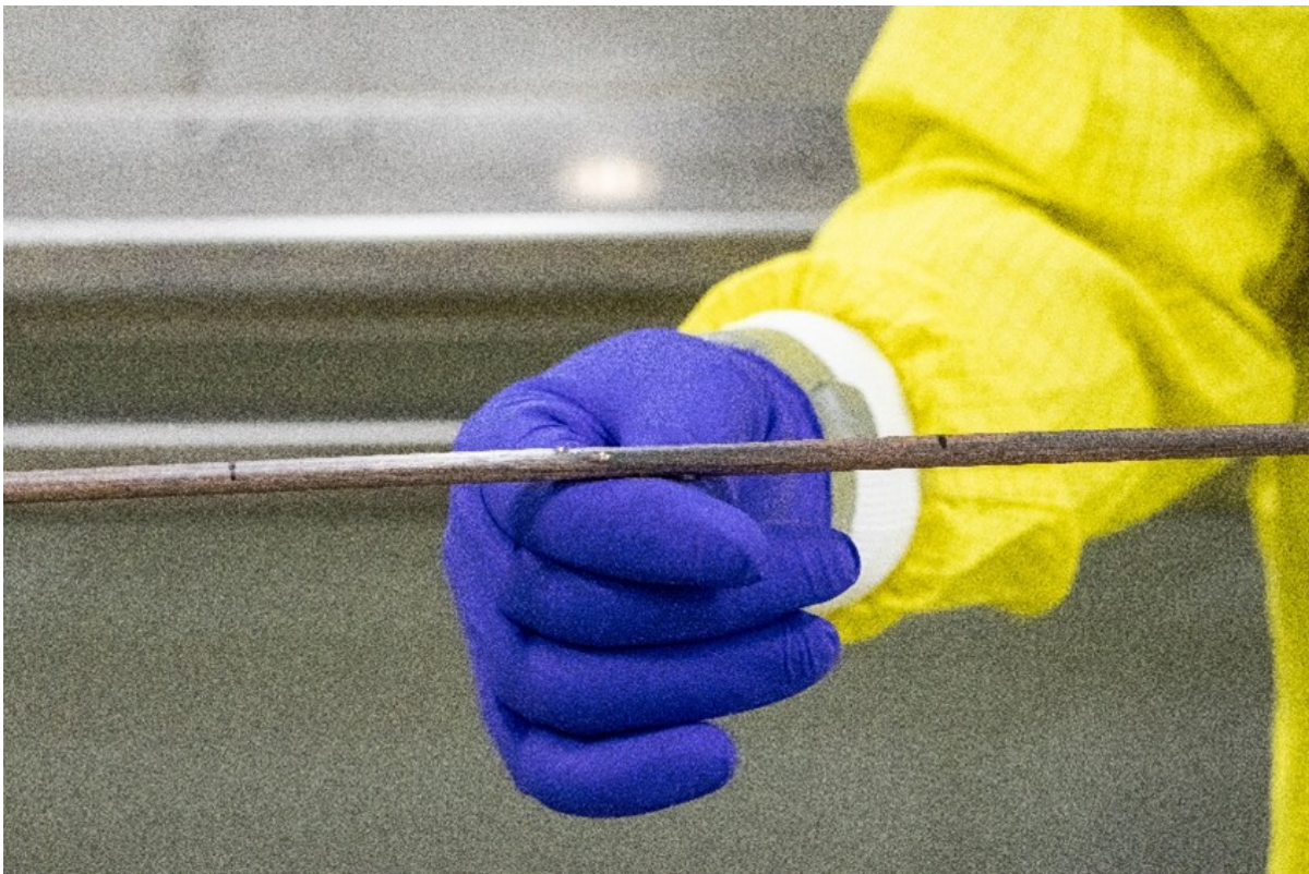
Image 2: Close-up View of the Enriched Uranium-Zirconium Rod Post-Extrusion, still covered in the extrusion lubricant
