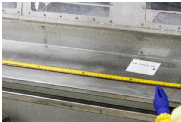
Taking Measurements of the Enriched Uranium-Zirconium Rod Post-Extrusion
