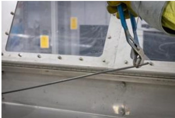
Co-extruded rod sample after co-extrusion process
