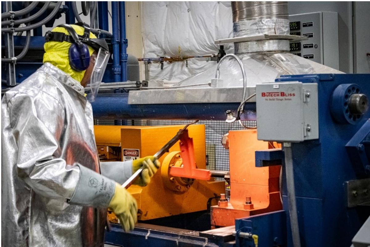
Figure 2: Heated-up billet assembly being loaded into the extrusion press prior to co-extrusion
