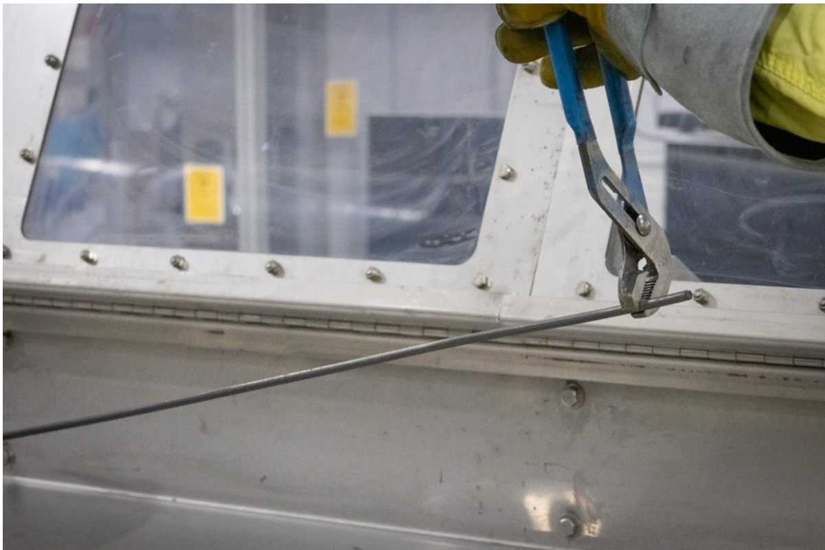
Figure 3: Co-extruded rod sample after co-extrusion process
