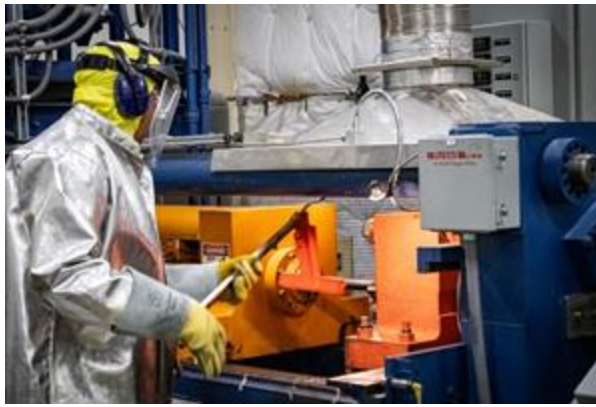
Heated-up billet assembly being loaded into the extrusion press prior to co-extrusion
