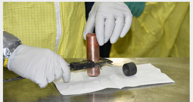
Taking Measurements of Billet Dimensions
