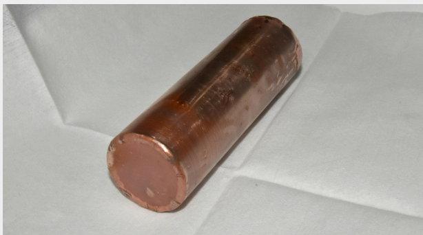
Uranium-Zirconium Alloy Billet Encased in Copper Sheath
