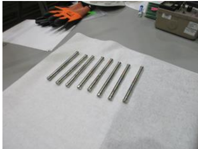
Capsules Containing Lightbridge Fuel Material Samples Before Loading into an Experimental Assembly
