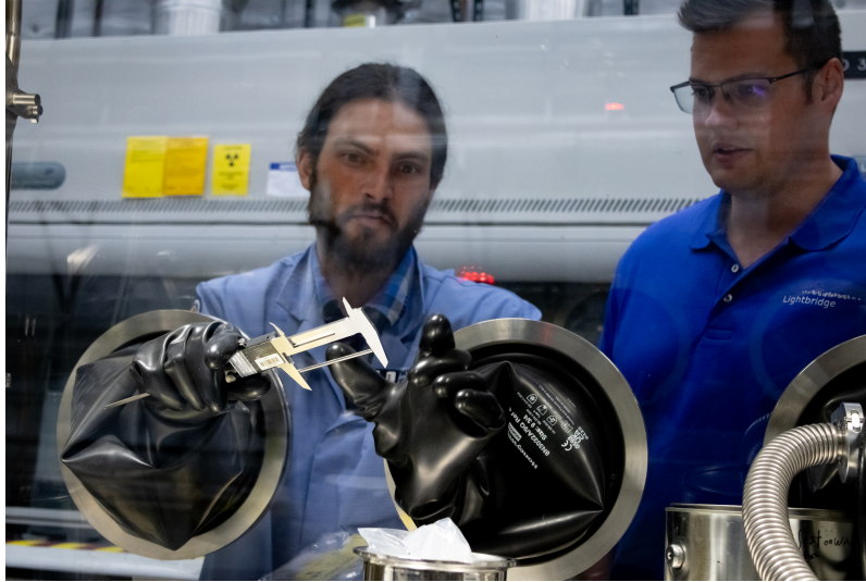
Image 1: Lightbridge and INL Team Performing a Visual Inspection of a Finished Enriched Uranium-Zirconium Coupon Sample inside a Glovebox
