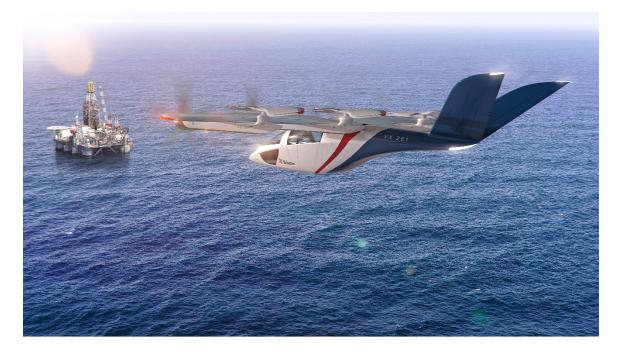
Vertical has developed the VA-X4, a piloted electric, zero carbon operating emissions, vertical take-off and landing (eVTOL) aircraft capable of carrying four passengers with a top speed of up to 200 mph (174 knots) and a range of 100+ miles (161+ kilometres).
