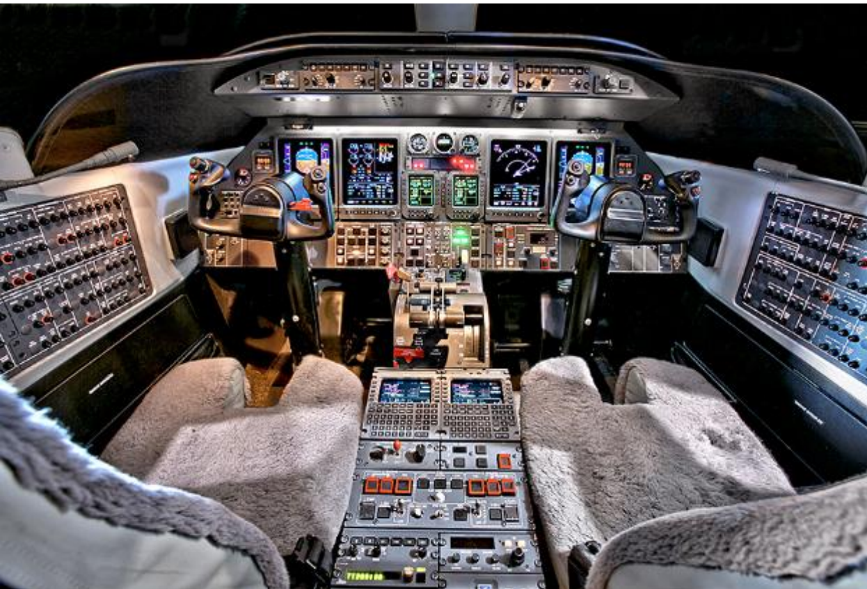
Traditional Cockpit with Mechanical Circuit Breakers Learjet 45
