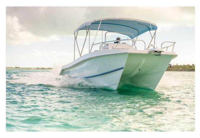
This Twin Vee catamaran has two hulls, widely spaced, each nearly at her beam ends, rather than a single monohull that is deep on the centerline
