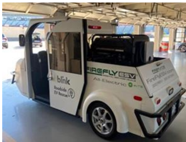
FireFly EV Roadside Assistance Vehicle with Blink IQ 200-M Mobile EV Charger
