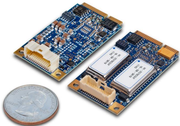
Miniature Ballard ME1000 avionics databus interface cards enable embedded computers and other systems to reliably communicate with and monitor ARINC 429/717 or MIL-STD-1553 equipment.
