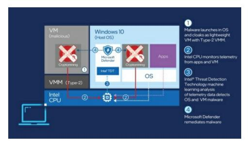
By leveraging Intel Threat Detection Technology , Microsoft Defender for Endpoint gains full stack visibility to detect advanced threats, such as cryptojacking, and can remediate the attacks before the user's PC is affected. (Credit: Intel Corporation)
