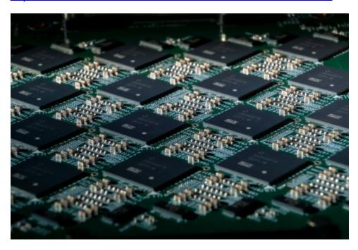
A close-up shot of an Intel Nahuku board, each of which contains 8 to 32 Intel Loihi neuromorphic chips. Intel's latest neuromorphic system, Pohoiki Beach, is made up of multiple Nahuku boards and contains 64 Loihi chips. Pohoiki Beach was introduced in July 2019. (Credit: Tim Herman/Intel Corporation)
