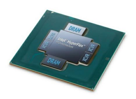
The Intel® Stratix® 10 MX FPGA is the industry's first field programmable gate array (FPGA) with integrated High Bandwidth Memory DRAM (HBM2). By integrating the FPGA and the HBM2, Intel Stratix 10 MX FPGAs offer up to 10 times the memory bandwidth compared with standalone DDR memory solutions. (Credit: Intel Corporation)
