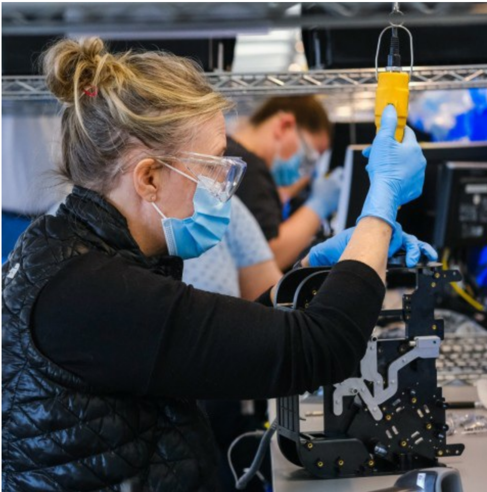
GM 3D printed tooling used for critical care ventilators on Stratasys systems. (Photo: Business Wire)
