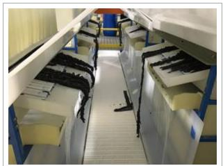
AquaRefining module with six electrolyzer units continuously producing AquaRefined pure lead, flowing like a waterfall of lead infused electrolytes
