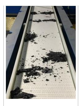
Conveyer belt carries pure lead to ingot casting area
