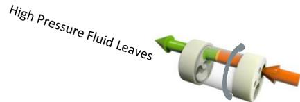
Cycle 3\* - Low pressure fluid in the ducts are exposed to high pressure fluid when ducts rotate and open to high pressure port
