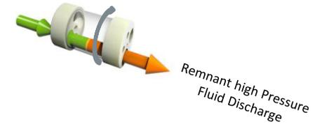
Cycle 1\* (Part 2) - Remnant high pressure fluid loses pressure as it opens to low pressure outlet port, as low pressure fluid enters from low pressure port.
