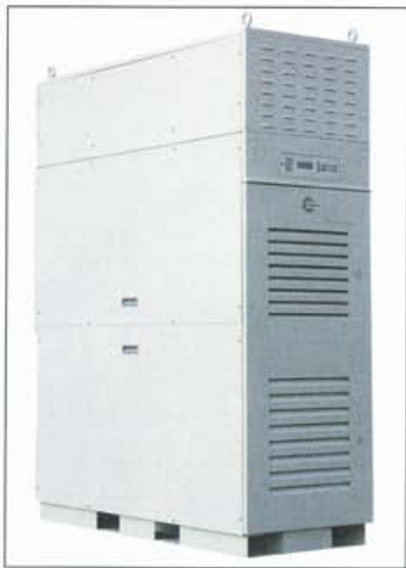
Figure 3: With trigeneration or Combined Cooling, Heating and Power (CCHP) applications, the heat output of Capstone C65 ICHP microturbines can be used to both heat and air condition a facility via absorption cooling
