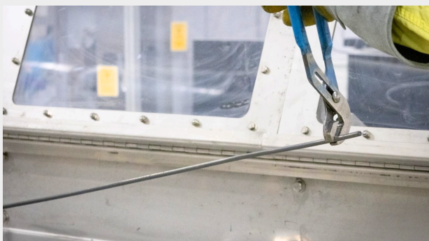
Co-extruded rod sample after co-extrusion process
