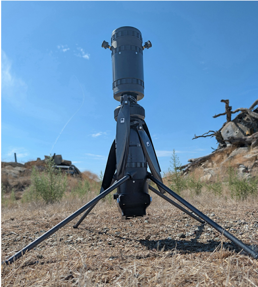
Robinson Unmanned SPIRIT™ Group 1 unmanned aircraft system (UAS) with MicroVision Movia™ Air Plus payload attached.
