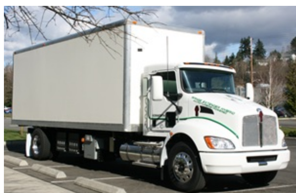
A Capstone C65 microturbine provides extended range by charging a 47kWh Li-Ion battery pack onboard.
