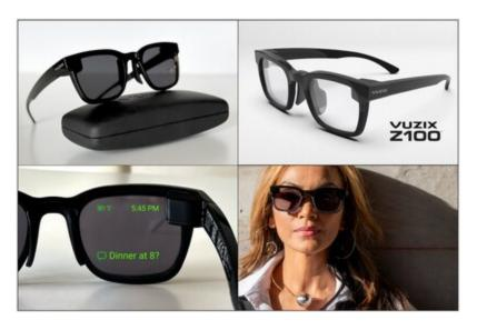
Vuzix Z100 smart glasses pack industry-defining heads-up waveguide technology into a sleek, fashionable form factor that weighs in at just 38 grams – the weight of a standard pair of glasses. Running up to 48 hours on a single charge, they deliver a crisp, transparent, monochrome image that can deliver important information hands-free while providing a natural AI delivery interface.
