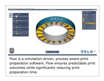
Flow is specifically designed for Sapphire, VELO<sup>3D</sup>'s laser fusion metal additive manufacturing system. It includes tools that help with part orientation, support generation, simulated print predictions, per-surface process application, slice composer and process review. As a result, manufacturers can now print complex part geometries SupportFree, enabling volume manufacturing of parts that are otherwise impossible or uneconomical to print due to hard-to-remove support structures.
