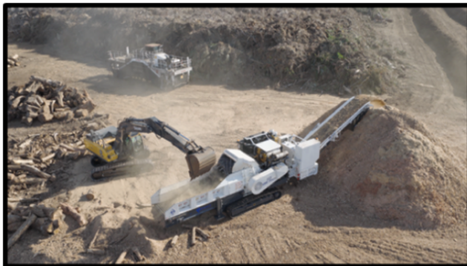
Diamond Z horizontal grinder operating at RenX's materials processing facility
