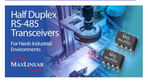
MaxLinear's new half-duplex serial transceivers offer small form factor packages, up to 50Mbps data rates, low EMI, IEC61000-4-2-ESD protection, and IEC61000-4-4 electrical fast transient (EFT) protection for harsh industrial environments. (Graphic: Business Wire)
