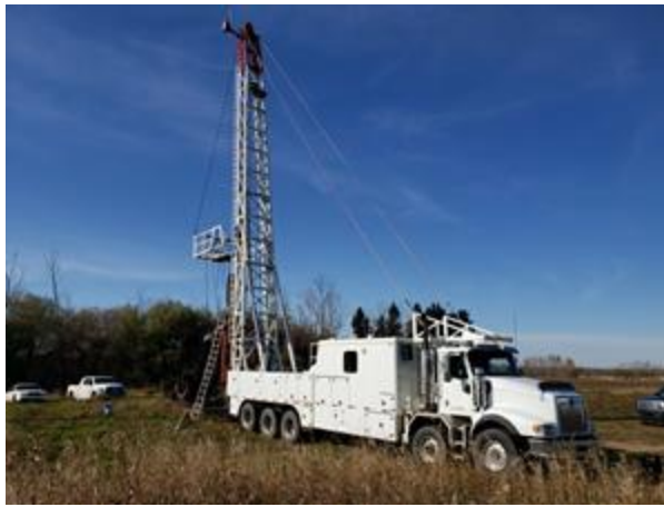
Olenox key combo service rigs and service support equipment on a well workover.
