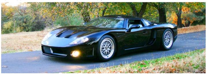
The Capstone CT-380 hybrid, based on a Factory Five sports car chassis, uses a 30 kw/40 hp turbine engine to provide power to charge its Li-ion battery pack.
