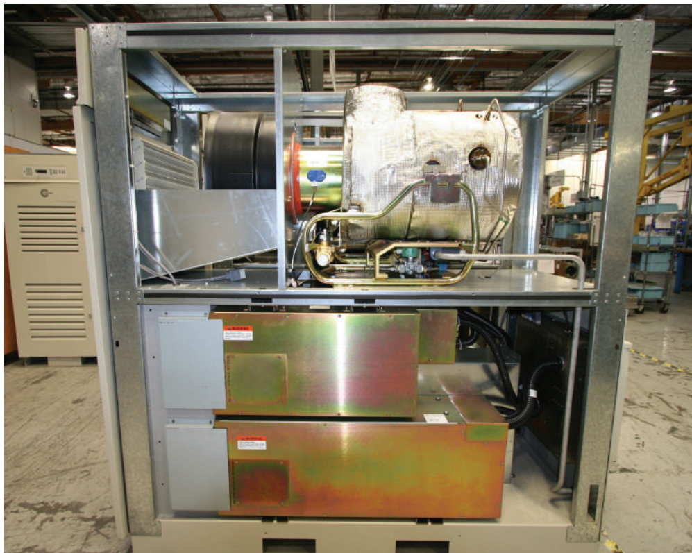
◀ Capstone C65 unit with panels removed. The systems are scalable from 30 kilowatts to several megawatts, and can run on natural gas, liquid fuels or renewables.
