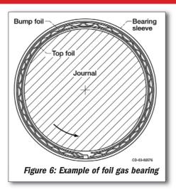
DellaCorte, whereas oil-lubricated bearings have film pressures of hundreds of psi. Therefore, foil gas bearings thrive on light loads and high speeds.
