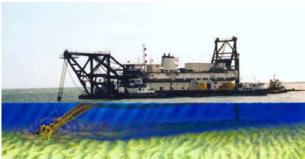
Figure 13. Illustration of cutter suction dredge
