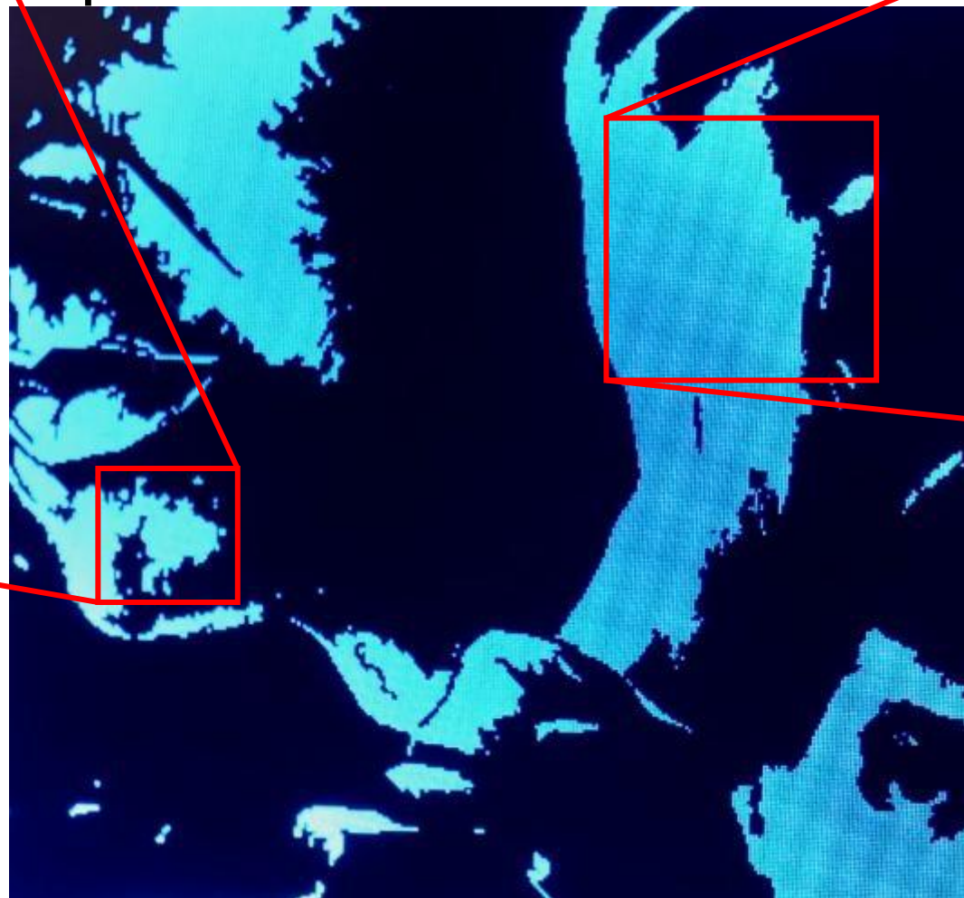
Approximately 27000 micro-LEDs with no observed faults
