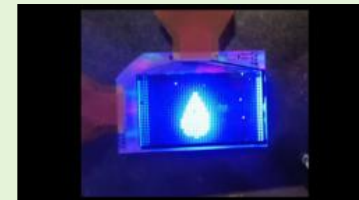
25ppi 27x48 OTFT-mini LED Backlight (2.17" diagonal)
