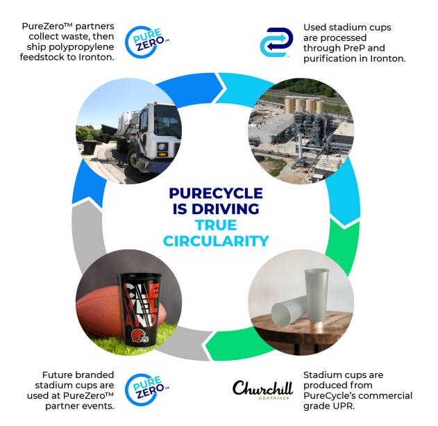
The PureCycle purification process is designed to transform polypropylene plastic waste into a continuously renewable resource. The first-of-its-kind technology removes color, odor, and other impurities from plastic waste, resulting in an ultra-pure recycled resin that can be recycled and reused multiple times.
