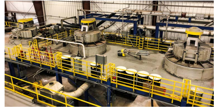
An additional kettle (far left) installed and operating with first metallic lead product shipped in March 2019 – will initially provide up to a 25% increase in ingot production and improve contribution margin.
